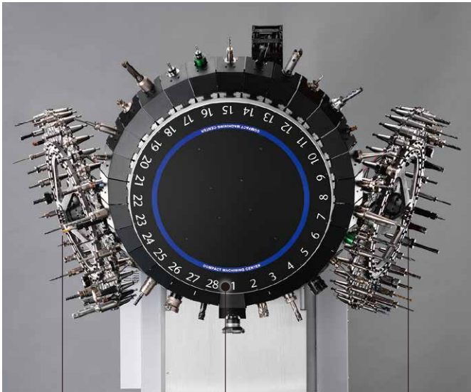
Left-side tool stocker Turret magazine Right-side tool stocker
